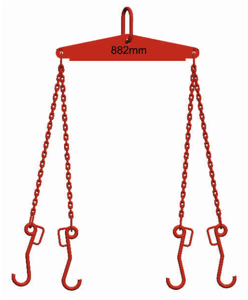
For MPCH Master Bushing 37.1/2" Figure No. 53
